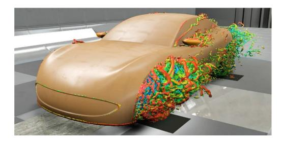
Simulation allows vehicle aerodynamic performance to be evaluated early in the design process, providing stylists insight to make design decisions without compromises.
