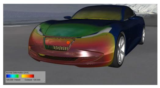
Crucially, by marrying creative freedom with the ability to optimize aerodynamic performance from the start of the design process, DesignGUIDE can rapidly accelerate vehicle development. Better communication between engineering and design teams, coupled with intuitive guidance, speed up the process of creating right-first-time designs that combine aesthetic with aerodynamic performance.
