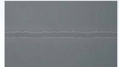
Figure 2 - 200 micron printed SU-8 feature
