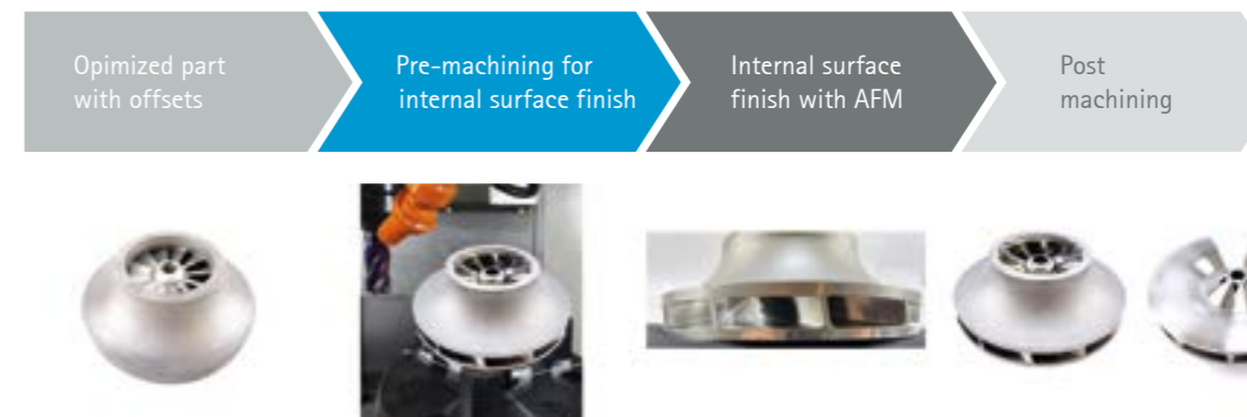
Figure 15: Manufacturing workflow for closed impellers
