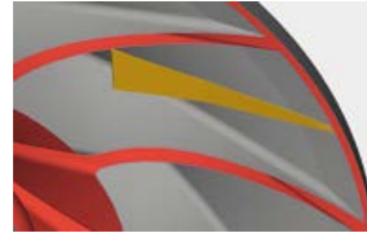
Figure 8: Bridging supports between blades
