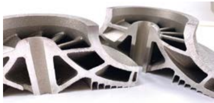
Figure 2: Cross section of a support-free impeller
