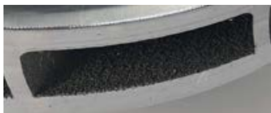
Figure 13: Downskin surface under the microscope and close-up view on downskin surface (15°)
