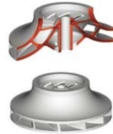
Figure 4: Cross section and side view of the designed impeller
