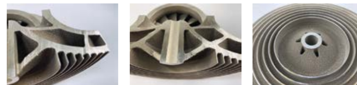
Figure 12: Images highlighting the as-built quality of the high energy downskin approach
