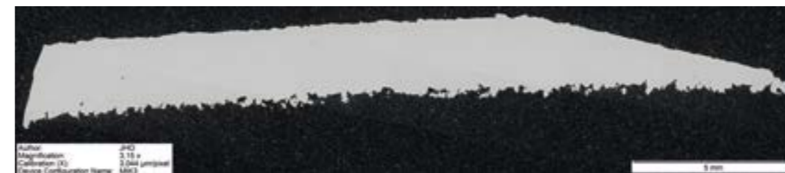
Figure 11: Crosscut high energy downskin exposure
