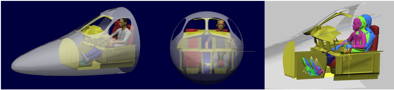
Figs. 1-3: Cockpit and passenger area design: vision, reachability, seat & space requirements
