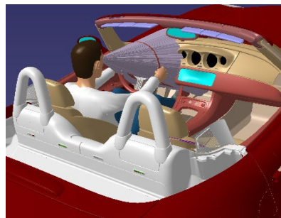
Fig. 1: Analysis of the direct visual field – the steering wheel rim is obscuring the view of the switch
