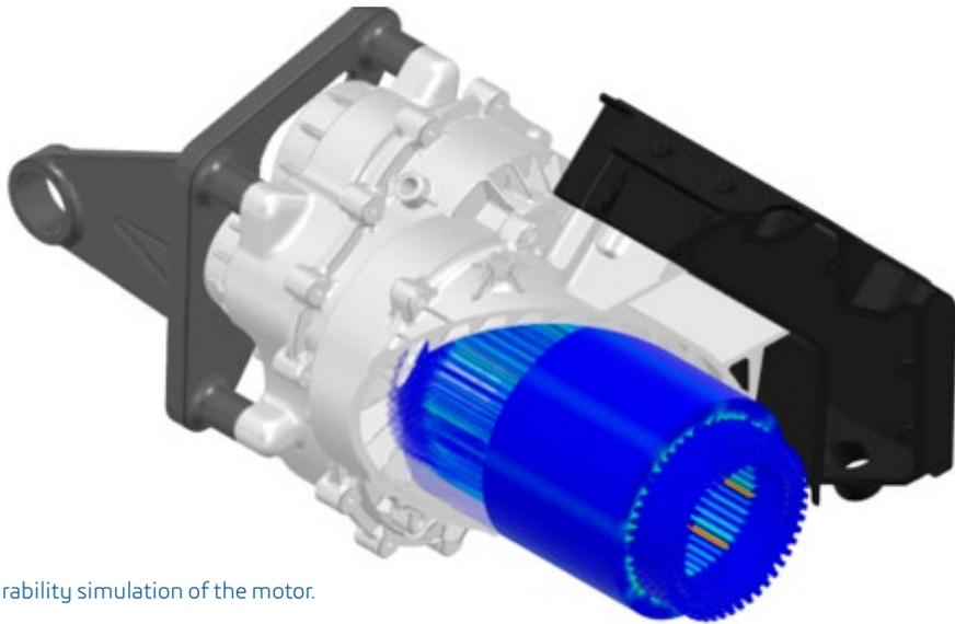
Durability simulation of the motor.
