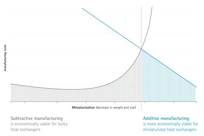
Figure 3: Delicate and complex components are where additive manufacturing shines, whereas massive parts with simple geometries are better suited for traditional subtractive manufacturing methods.
