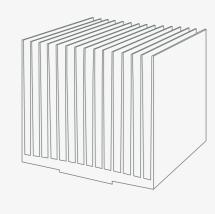
Figure 2b: Complex water cooler assembled from sub-components made by different conventional manufacturing techniques
