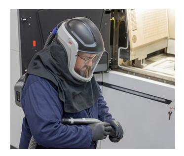
For respiratory and face shielding needed to operate an metal AM system during certain steps, we recommend the **3M Versaflo Heavy Industry PAPR Kit TR-300-HIK**. In the accessories kit that is provided with a metal system purchase, there is one welding cape included. If there is an additional technician aiding in a filter change, they will need one for flash protection as well.
