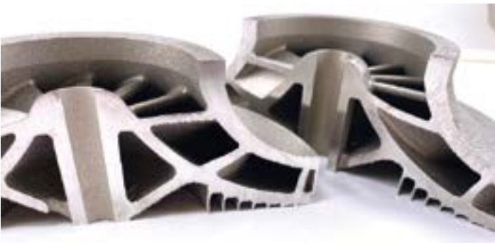
Figure 2: Cross section of a support-free impeller
