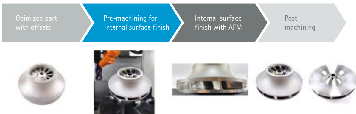
Figure 15: Manufacturing workflow for closed impellers
