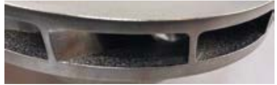
Figure 18: Detailed view of downskin surface after AFM
