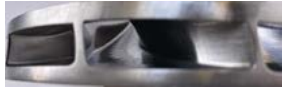
Figure 17: Detailed view of upskin surface after AFM
