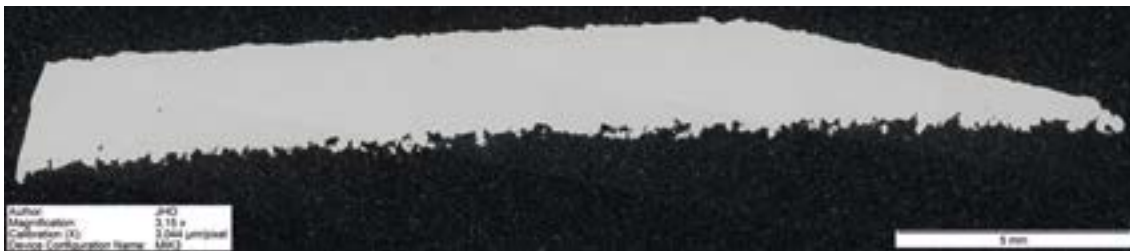
Figure 11: Crosscut high energy downskin exposure
