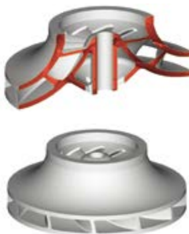
Figure 4: Cross section and side view of the designed impeller
