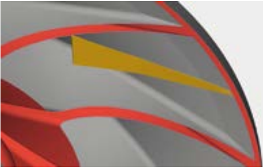
Figure 8: Bridging supports between blades
