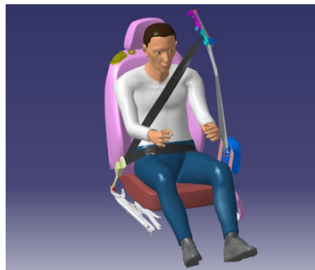
Fig. 1: Analysis of ergonomic belt routing
