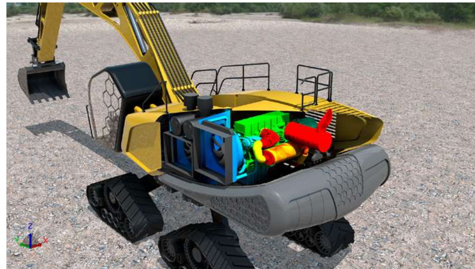
Key-off underhood simulation, ensuring robustness of design
