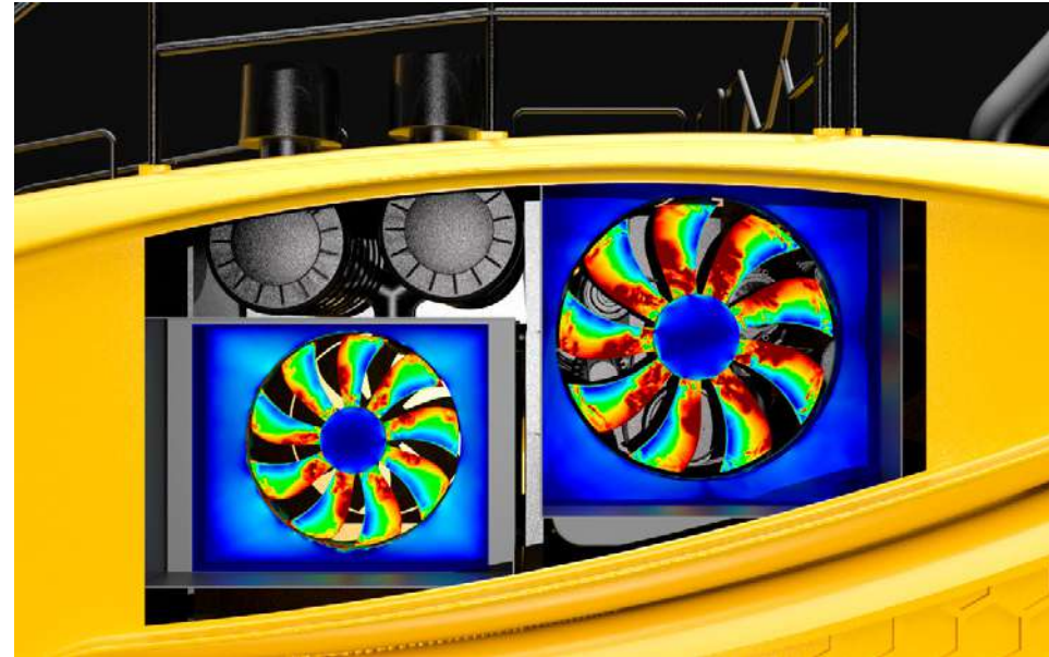
Double underhood fan noise simulation
