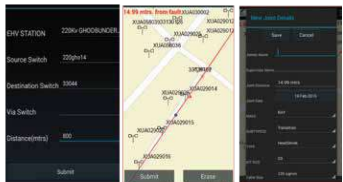
Fig 3: Fault Locator App on Mobile
