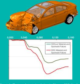
Frontal offset crash test simulation in Abaqus FEA (top) and corresponding firewall intrusion results with and without local failure mechanisms incorporated in the model (bottom).
