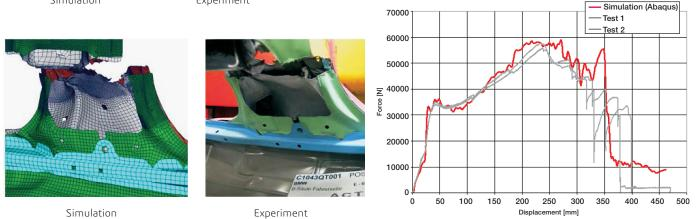
deployment in production design simulation. Leveraging realistic simulation to achieve such accurate local predictions within global design models early in the vehicle program increases vehicle design development efficiency by avoiding problems later, when changes are more costly to correct and can impact vehicle launch timelines.
