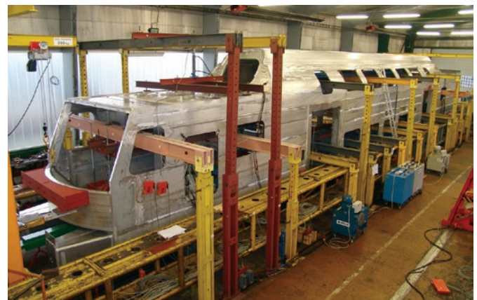
Figure 4: Full-size railcar body set up for static testing
