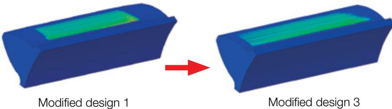
Optimizing gears with Isight resulted in a design that lowered contact stress across the entire surface.
