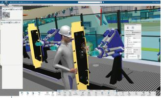
Different **3DEXPERIENCE** applications were used to simulate the future wing production line (for example, Ergonomics at Work application was used to study operators workstations layout, reachstudies, and ergonomics). Robot and equipment simulation was used to demonstrate the assembly processes of the wing structure and equipment.
