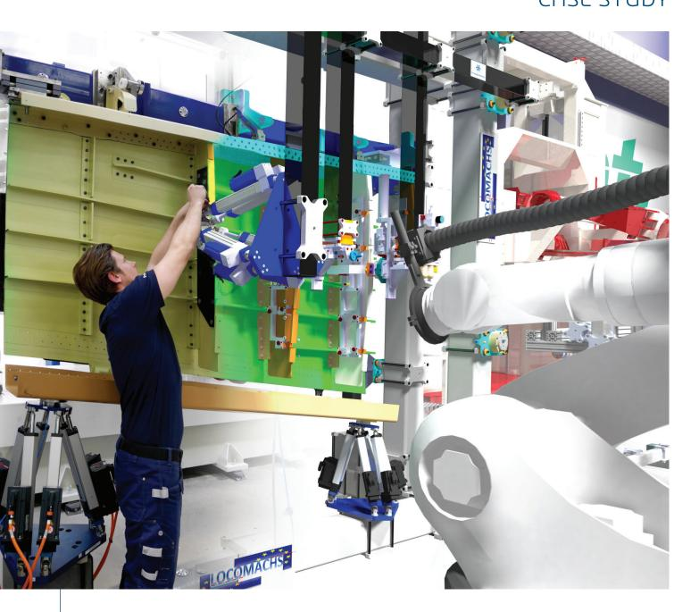
The LOCOMACHS physical demonstation fixture is built with reconfigurable tooling and simulated in **3DEXPERIENCE®** to fully demonstrate and test key technology enablers for future wing production. Peter Helgosson (pictured) demonstrates a virtual to real image of the demo cell ("Digital Twin").
