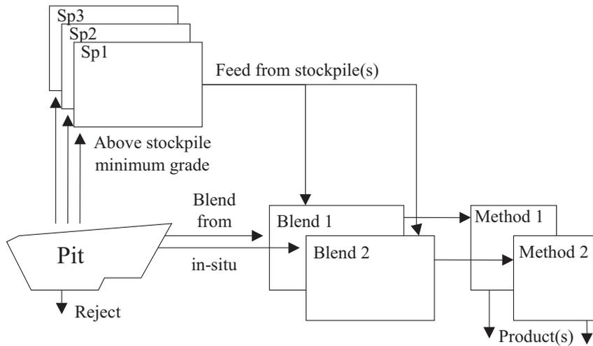
FIG 1 - Extractive blend schematic.
