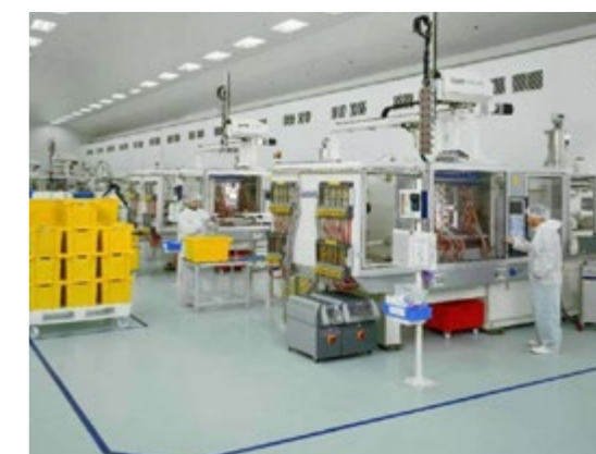
Figure 9: Production line for an inhaler. The set-up is usually in operation for over ten years.
