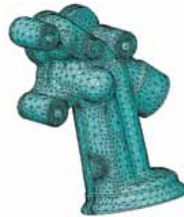
Model for an oil filter adaptor NVH (noise, vibration, and harshness) analysis.
