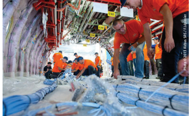
With CATIA, Airbus implemented a full 3D Master approach to design the electrical harness installation for the A350 XWB. Any errors were corrected digitally before physical installation.
