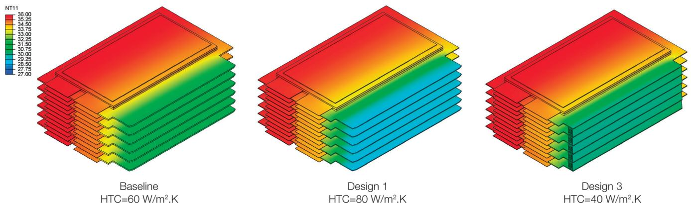
Figure 2. Abaqus FEA models of stabilized cell temperatures for three module designs with similar steady state temperatures. Compared with the baseline, Designs 1 and 3 are smaller. However Design 1 requires higher air flow.
