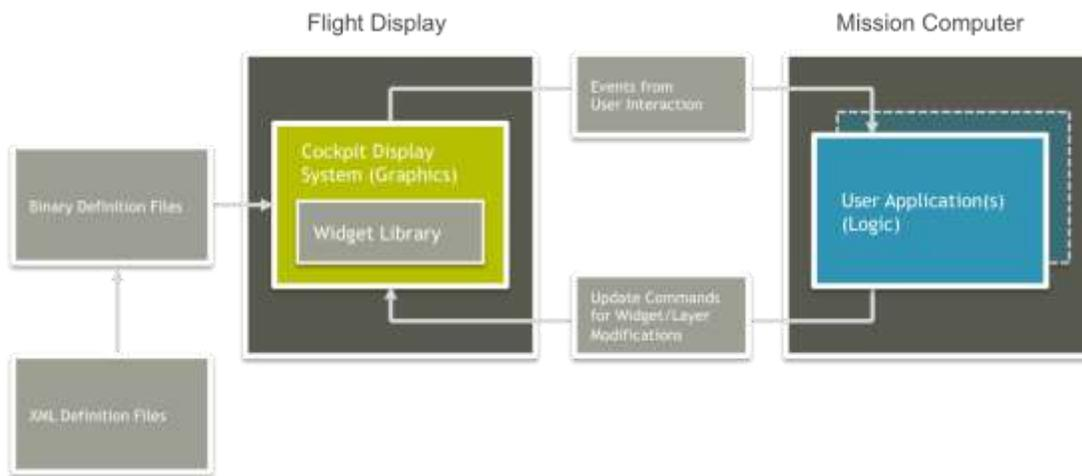
Besides being a simple recipient, layers also have runtime properties that can be modified such as their visibility and activation state. When a layer is invisible, all of the contents will not be seen on-screen. When a layer is inactive, none of the widgets that it contains will be selectable.
