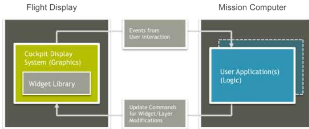
The aim of ARINC 661 is to minimise the impact on the user interface redevelopment and certification cost in response to inevitable system changes and deployment variations. In order to achieve this, all systems (UAs) need to “speak” ARINC 661 when interacting with the CDS. How UAs communicate amongst themselves is not affected.
