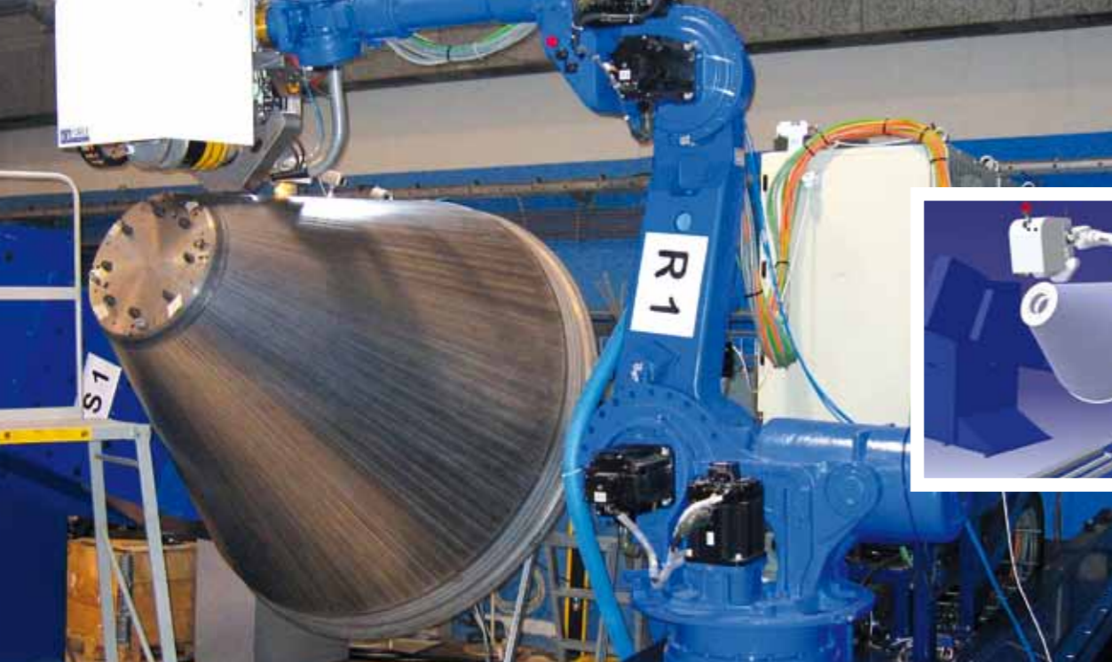
Robot inspects and welds sandwich cone structure
